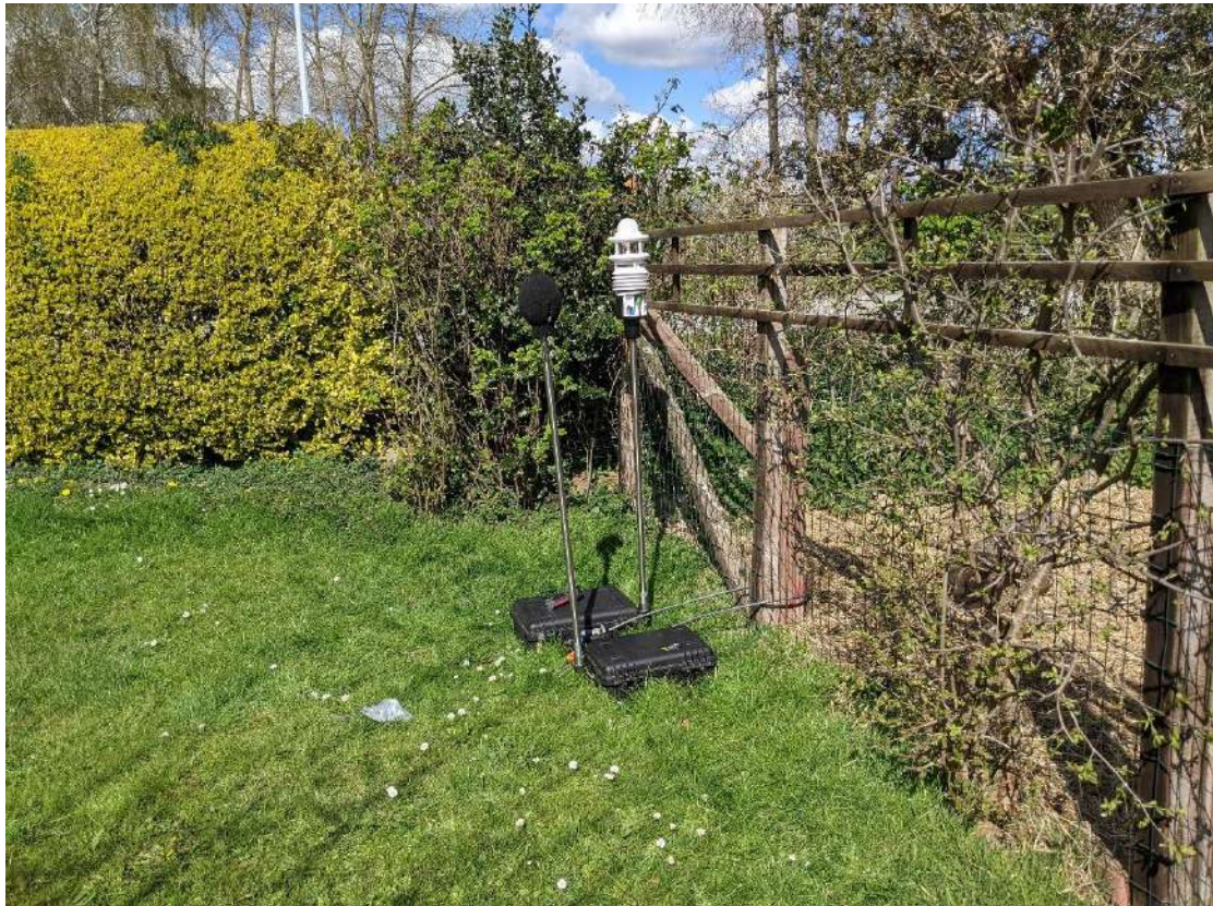
Figure 12: Noise Monitoring Setup at Charmaine, Amcotts
