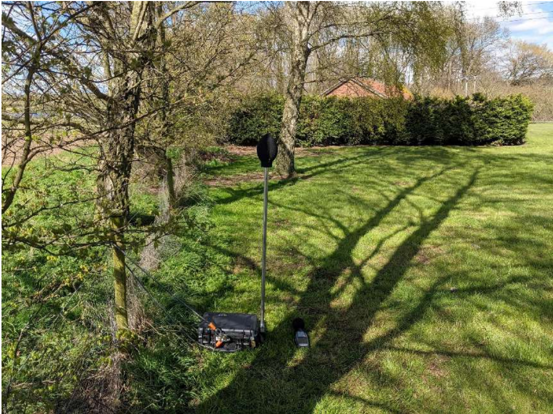
Figure 17: Noise Monitoring Setup at Park Ings Farm
