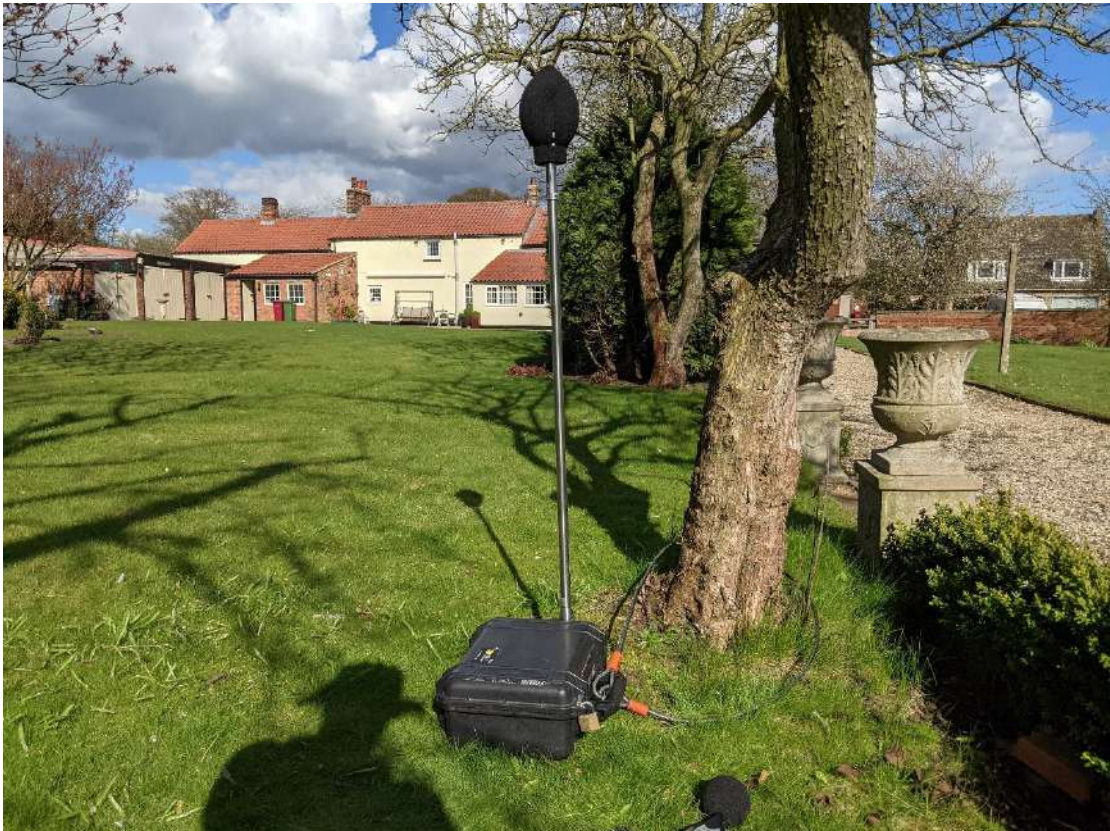
Figure 7: Noise Monitoring Setup at the Forge, Flixborough
